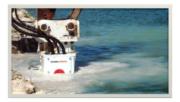
Drum cutters use a low energy method of impact resulting in low noise and vibration. Production rates are relatively high compared to hydraulic breakers, particularly in softer materials.
